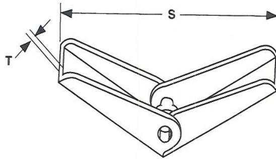
**Toggle Wings are a four-piece fastener consisting of two matching steel wings, an internally threaded nut, and a wire spring providing the necessary tension to open and close the wings.**
